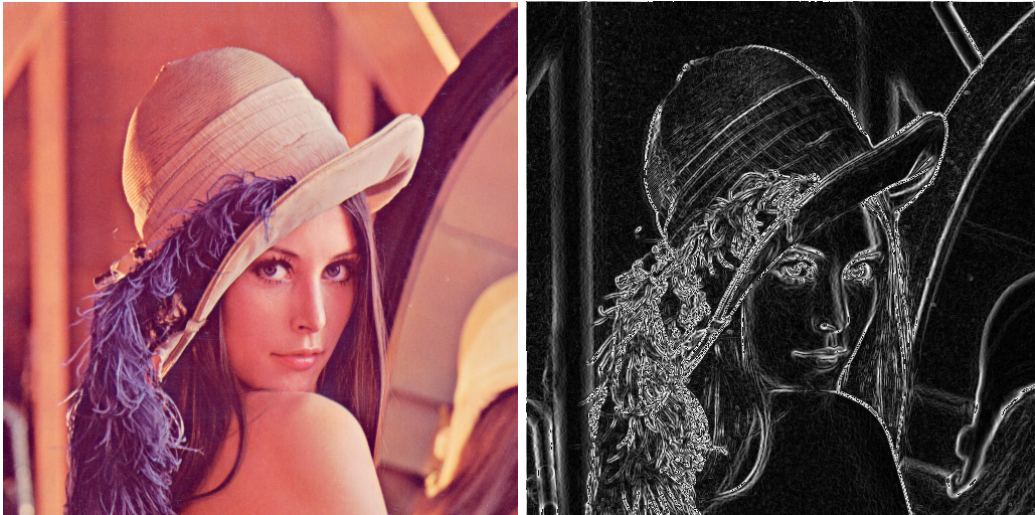
(a) Input RGB image I of the Sobel Filter (b) Application of the Sobel Filter onto I
