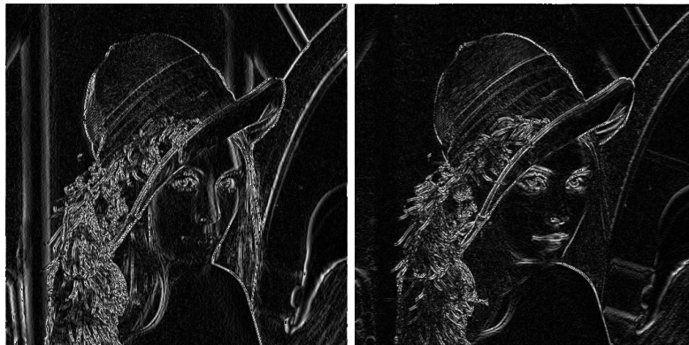
(a) Horizontal gradient G_x resulting from phase (2) of Section 1.1. G_x increases in the "right" direction. (b) Vertical gradient G_y resulting from phase (3) of Section 1.1. G_y increases in the "down" direction.
